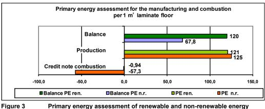
ure 3 Primary energy assessment of renewable and non-renewable energy sources for the manufacturing and combustion of 1 m<sup>2</sup> of laminate flooring.
