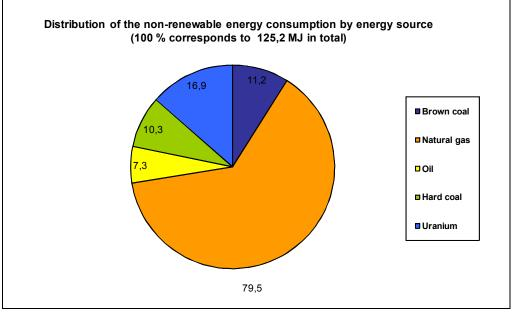
Figure 1: Distribution of the non-renewable energy consumption by energy source for the production of 1 m<sup>2</sup> of laminate flooring
