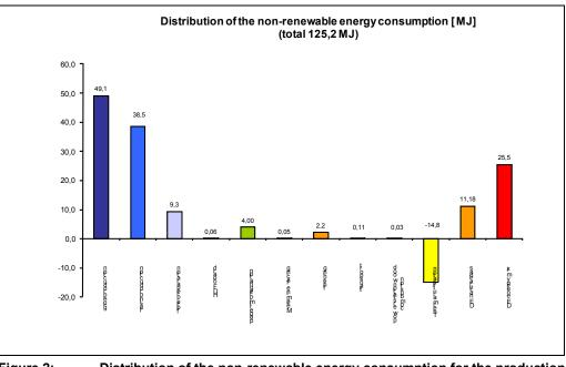
Figure 2: Distribution of the non-renewable energy consumption for the production of one square meter of laminate flooring.
